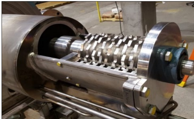
Developed and Validated New Auger-Grinder During Demonstration Run 1
