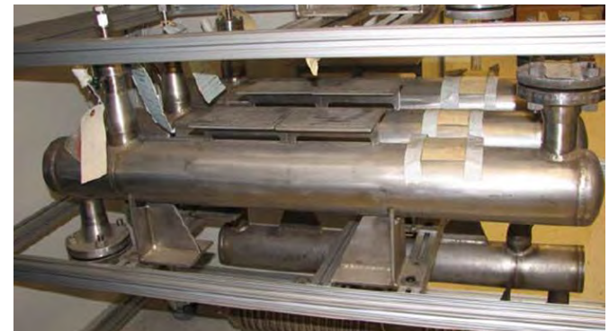
Existing Hydride Bed Stages shown above (14 will be replaced)
