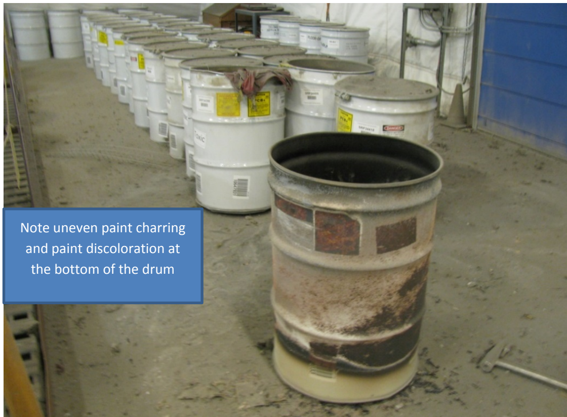
Figure 4. Drum 10648033 post-event exterior.
