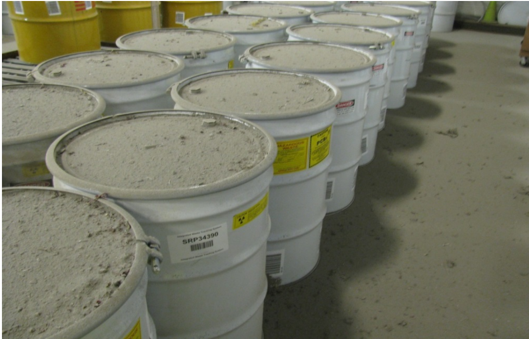
Figure 2. Ejected waste material on lids and floor.
