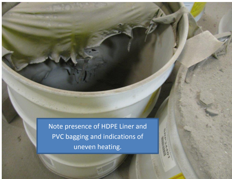
Figure 8. Drum 10647918 post-event interior.
