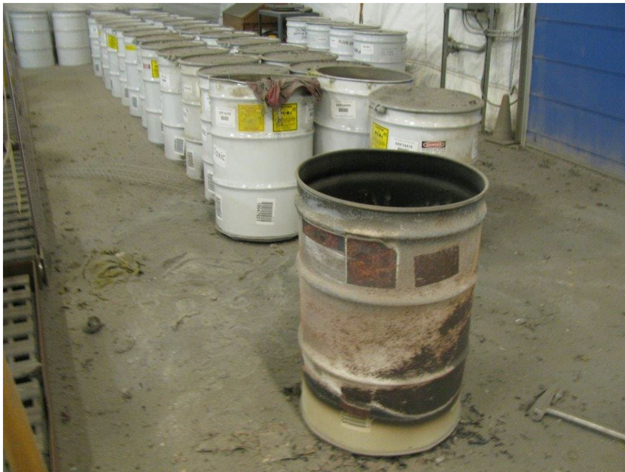
Ruptured waste drums at Idaho National Laboratory.
