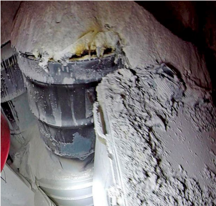
Drum of inappropriately remediated nitrate salt waste that reacted in the underground of the Waste Isolation Pilot Plant.
