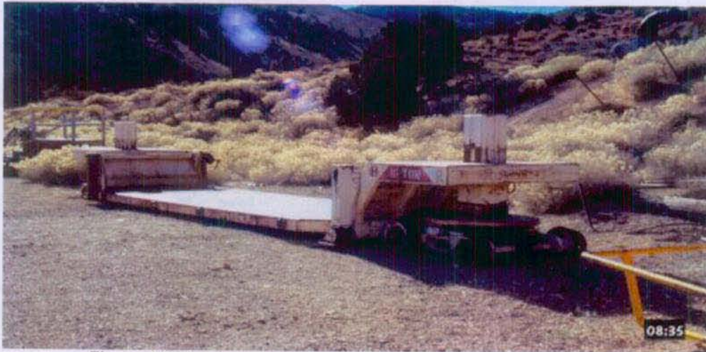
Figure 4-5. Lowboy to support movement of equipment and material.
