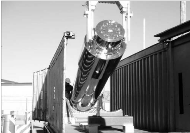
Cask is returned to its shipping container after being loaded
