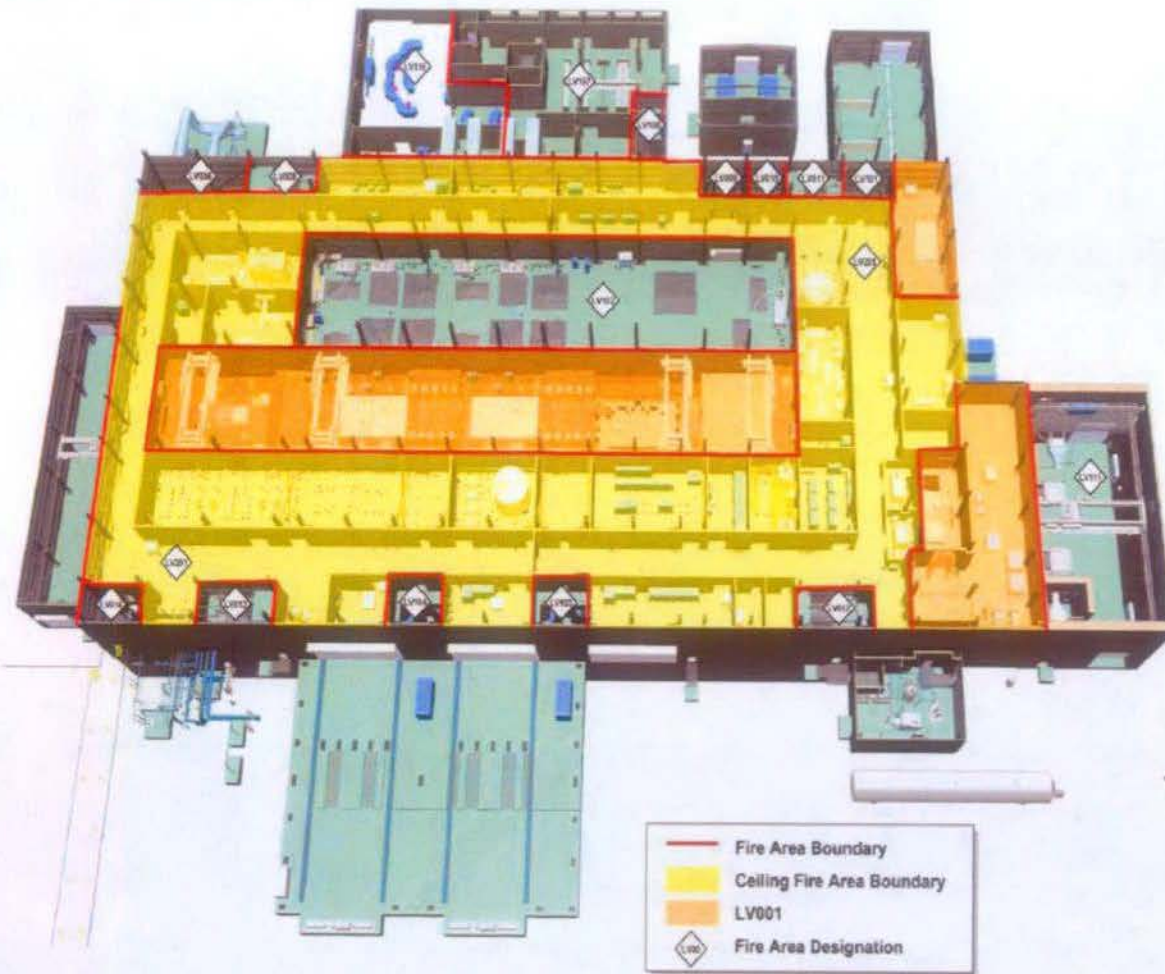
Figure 8 LAW Building Fire Boundaries at Elevation 28 Ft
