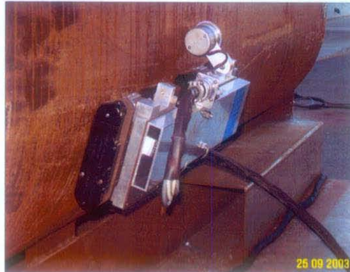
Figure 6: EMAT System for Guided Wave Inspection of Double Shell Tank Mock-up
