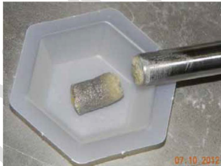
Figure A-3 Campaign 2, core sample 20-2 taken from the North mound after Cycle 10,
