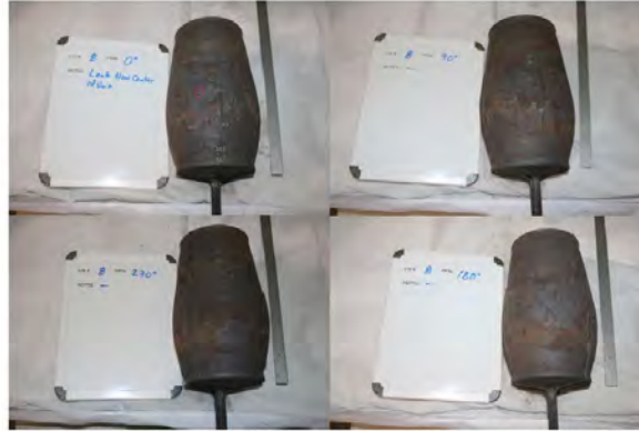
Figure 4-19. Post-test conditions of test vessel for Sequence 8. Angle positions refer to the visible portion of the vessel (see Figure 2-4). Angular positions, in clockwise direction, starting from upper left quadrant: 0°, 90°, 180°, and 270°.
