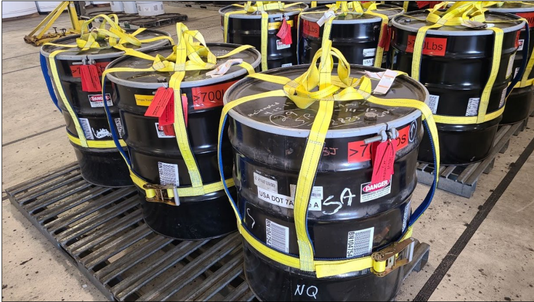
Figure 15. Lid Restraints on Drums with Flammable Gas
