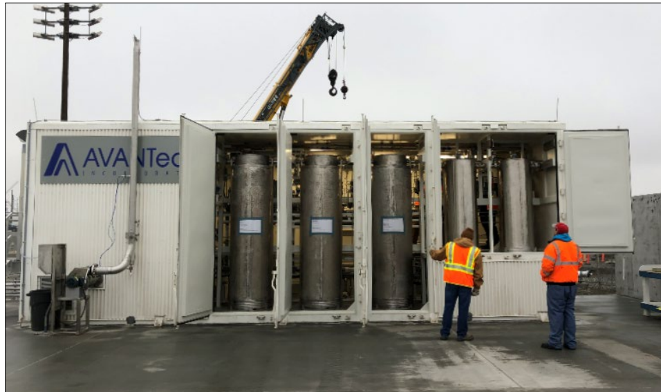
Figure 12. Tank-Side Cesium Removal Enclosure with Doors Open, Showing Ion Exchangers and Process Filters
