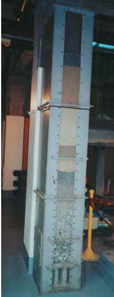
Figure 3. A vertical slice of a sand filter design used at the Hanford Site. Air enters the bottom and rises up through the sand filter media. The bottom layers of the sand filter media are composed of course rock with subsequent layers made of smaller material followed by a cap layer at the top.
