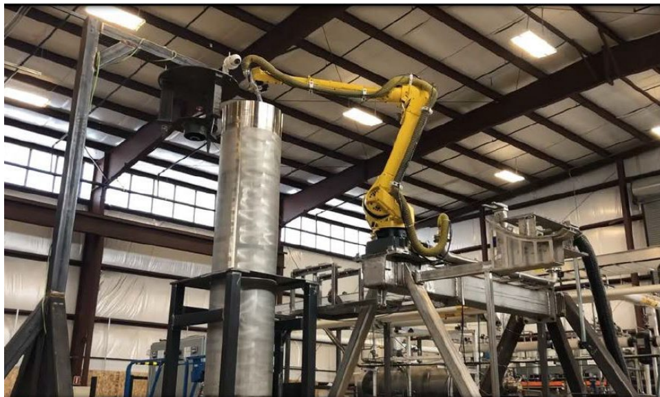
Full-Scale Mock-up of Canister Decontamination Testing
