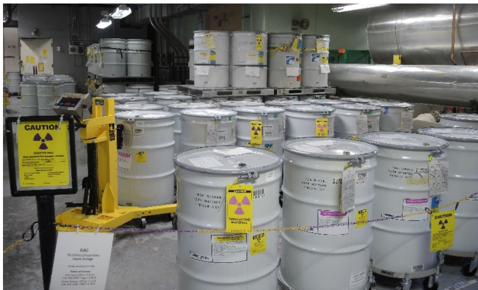
Transuranic Waste Containers Staged Inside the Plutonium Facility
