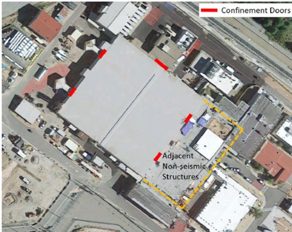
LANL Plutonium Facility Showing Confinement Doors
