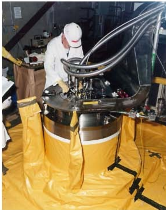
Cover Photograph: Nuclear Chemical Operators Attach Hoses to Ports in the Top of a Multi-Canister Overpack Holding 290-300 Irradiated Fuel Assemblies from Hanford's K-Basins, in the Cold Vacuum Drying Facility.
