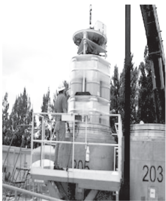
Lawrence Livermore National Laboratory Decontamination and Waste Treatment Facility are loading drums with radioactive waste into a TRUPACT II container for shipment offsite.
