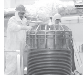
Workers at Paducah preparing a Cask from the L-Area to be transported to the E-Area for final disposal.
