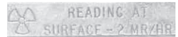
Actual caption from a fuel enrichment capsule from the Molten Salt Reactor at the Oak Ridge National Laboratory.
