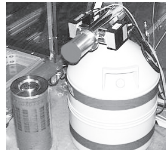
Savannah River has developed instruments to precisely measure quantities of nuclear material used to maintain accountability and control of strategic materials.
