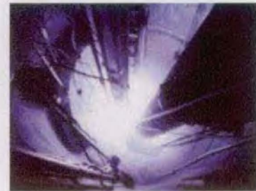
Cherenkov Radiation Is Seen as a Flash When the Annular Core Research Reactor Performs a Pulse
