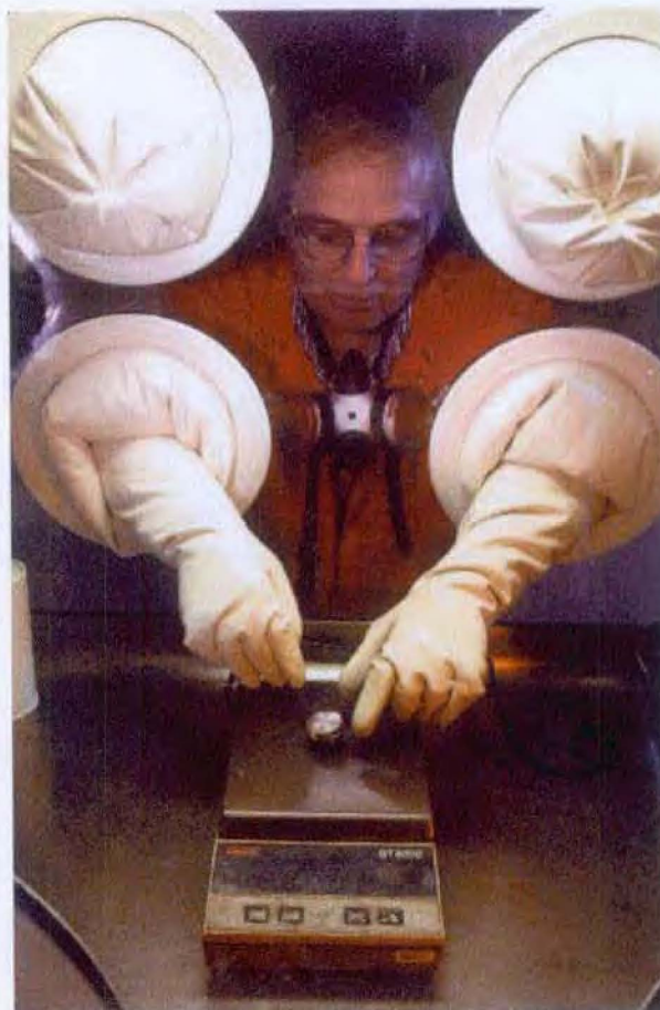
Machinist Bill Poulos, a Trained Fissile Material Handler, Weighs a Machined Plutonium Part in a Glovebox in the Plutonium Facility's Radioactive Materials Area. He is Using a Certified Balance That is Part of the Plutonium Accountability System. (Photo Credit: LLNL)
